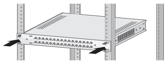
Figure 5. Securing the Power Supply with Screws
